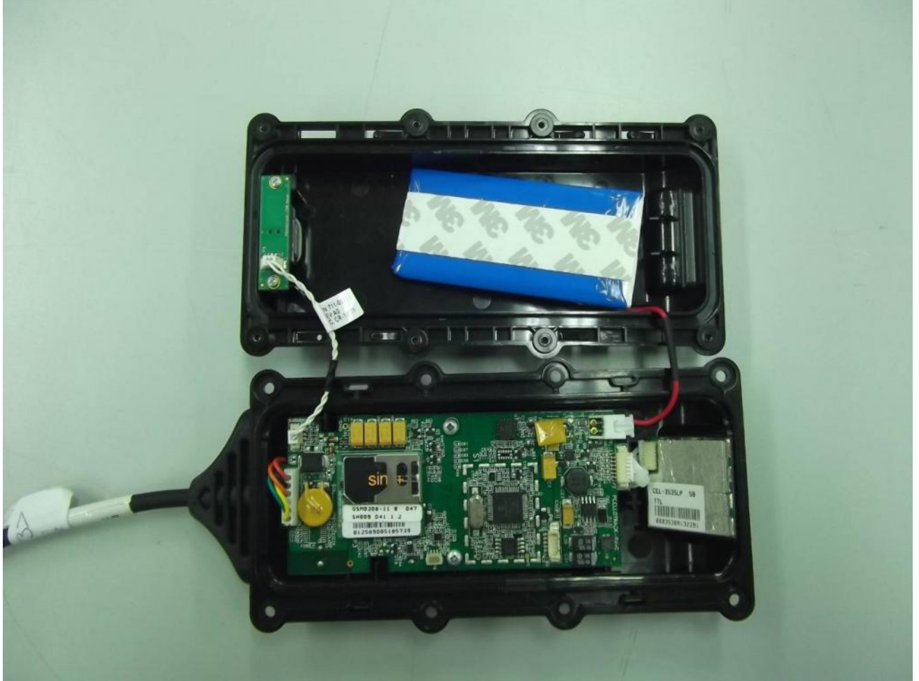
Picture 5. Internal View – Yoku battery
